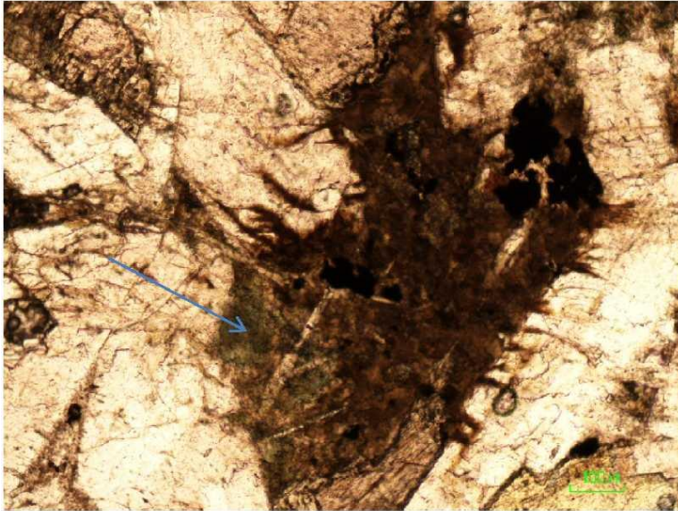
NL 2/9 _ 4.3–4.58: Secondary chlorite, an alteration product, distinguishable by its green colour. (x10 magnification, field of view 1250µm wide, plane polarized illumination)
