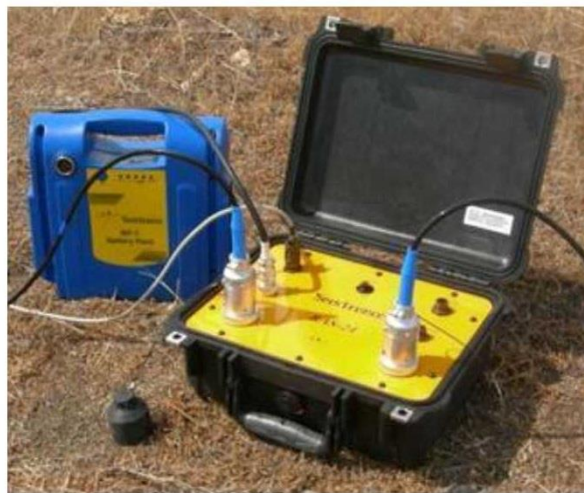
Figure 2. The seistronix Ras-24 seismograph with a battery source connected to it.
