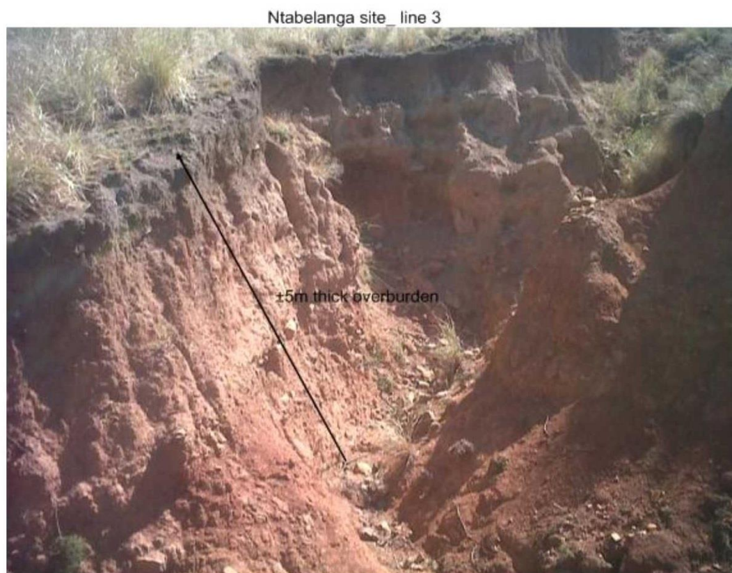
Figure 12. An image showing the relative depth extend of the thick overlying material, some dark grey-brownish colluvium and highly metamorphosed sandtones in an exposure zone along the position of line 3.
