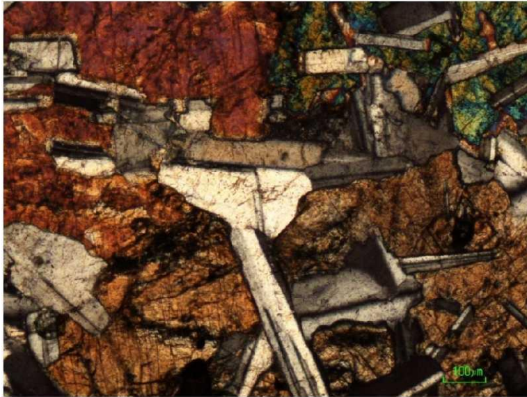
N1_ 11.84-12.2: Plagioclase showing polysynthetic twinning, enclosed by clinopyroxene.
