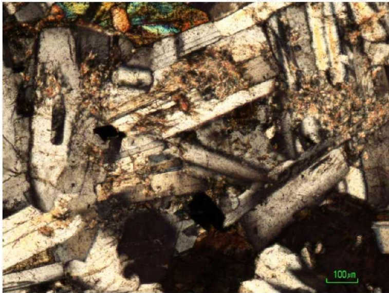
N1_ 11.84-12.2: Alteration of plagioclase to sericite (white mica)
